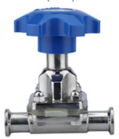
Sanitary diaphragm valve is SS304 or SS316L material. Sanitary designed with complete drainage of fluid. It can be sanitized in line with steam (SIP or CIP) or autoclave. It also allows precise control of the fluid flow rate with low turbulence and minimal back pressure.
